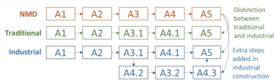
Figure 2 Module A of the MPG calculation according to the NMD and as applied in this study
