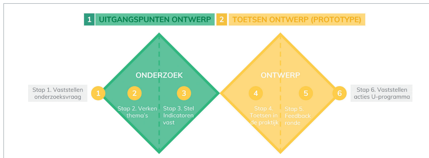
Figuur 3 De Double Diamond-methode (aangepast van Design Council (2005)).
